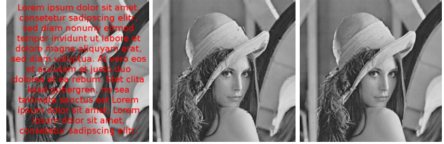
Figure 10: Left: Text degraded image, PSNR = 14.03dB Middle: Reconstruction using pre-defined DCT dictionary, PSNR = 30.9dB Right: reconstruction using KSVd learned dictionary, PSNR = 33.09dB
