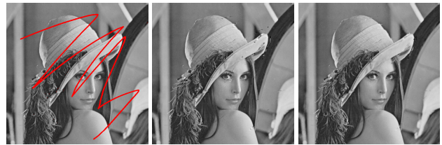
Figure 11: Left: Scratch degraded image, PSNR = 19.09dB Middle: Reconstruction using pre-defined DCT dictionary, PSNR = 33.68dB Right: reconstruction using KSVd learned dictionary, PSNR = 35.94dB
