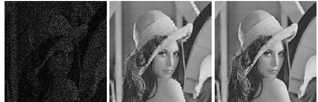
Figure 12: Left: Degraded image with 80% pixel loss, PSNR = 6.42dB Middle: Reconstruction using pre-defined DCT dictionary, PSNR = 24.27dB Right: reconstruction using KSVd learned dictionary, PSNR = 26.75dB
